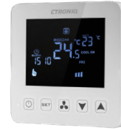
Smart Thermostat (CSST70) - 0.3W Power Consumption - 16A/250V Load Capacity - 5 °C - 35 °C Range - Switch relay - 1 week cycle - Weekly programming
